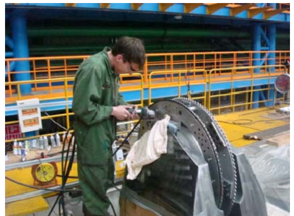
Goltens In Situ Machinist machining damaged Journal
