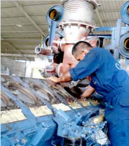
Cleaning of block liner bore
