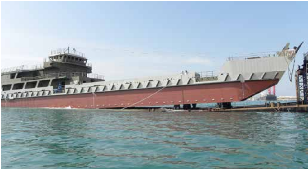
Afloat barge launch of the Al Shareeah (75 meter Roll on-Roll Off Landing craft)
