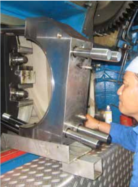
Removal of big end bearing housing
