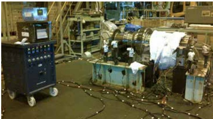
Annealing equipment set up on trial shaft in Yokohama
