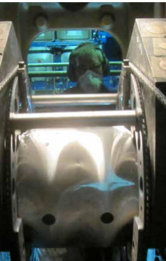
In-Situ Machining of the annealed crankpin in progress
