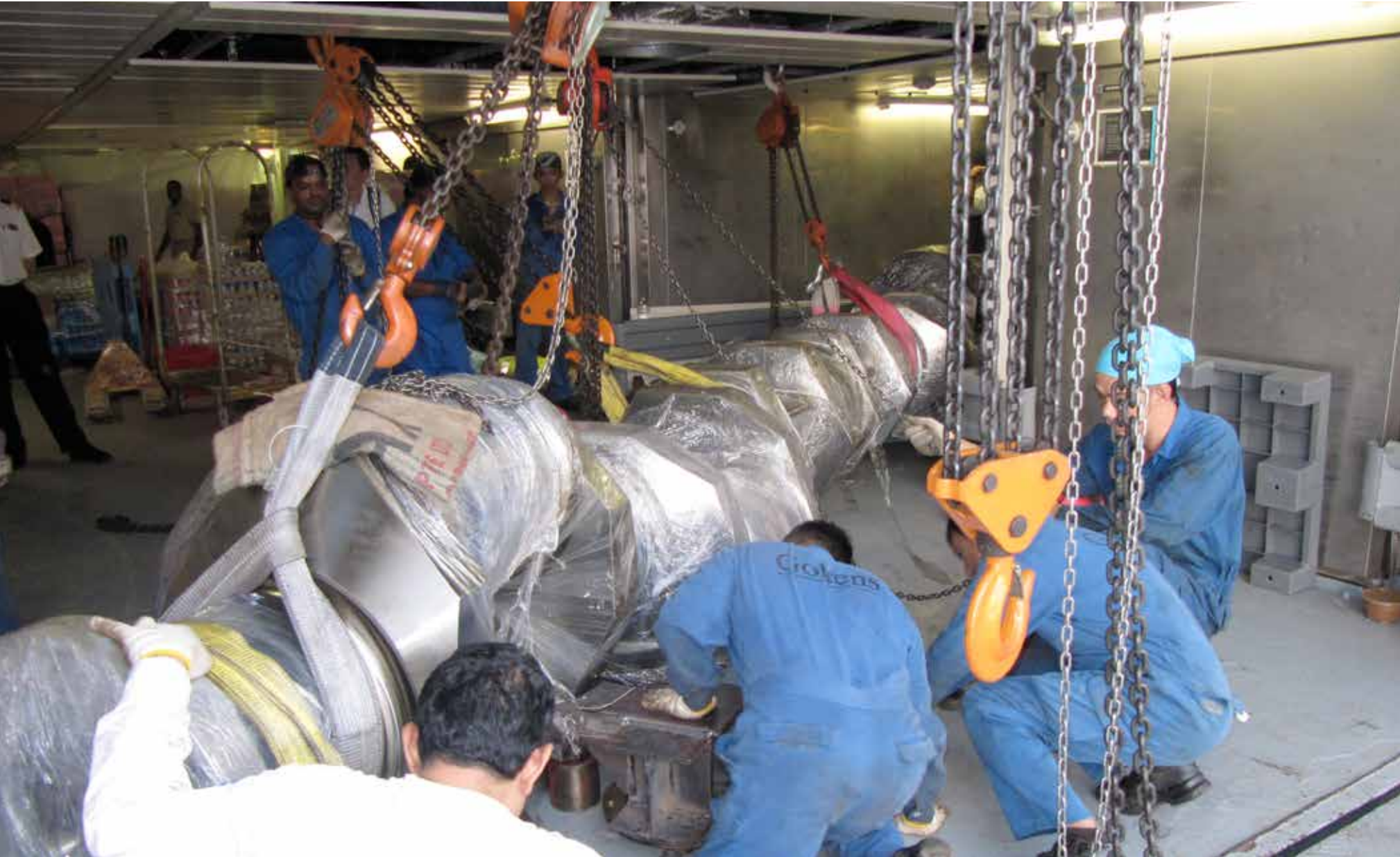
Preparing crankshaft for transport down passageway via skid
