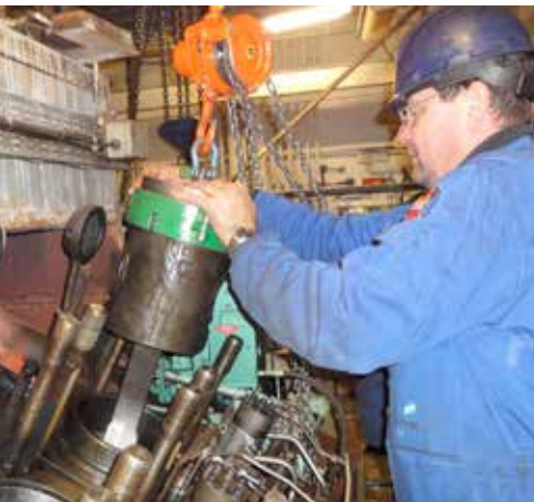
Reassembly of one of the overhauled pistons and connecting rods
