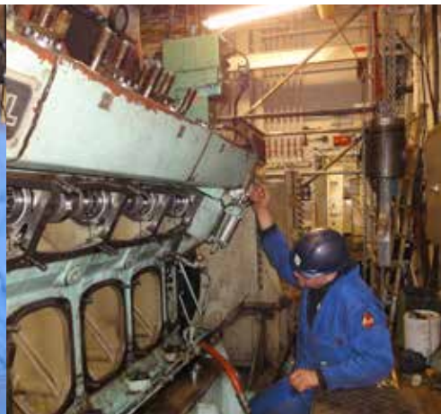
Rotating the engine to its correct position
