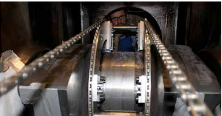
Post Annealing machining of the crankpin journal
