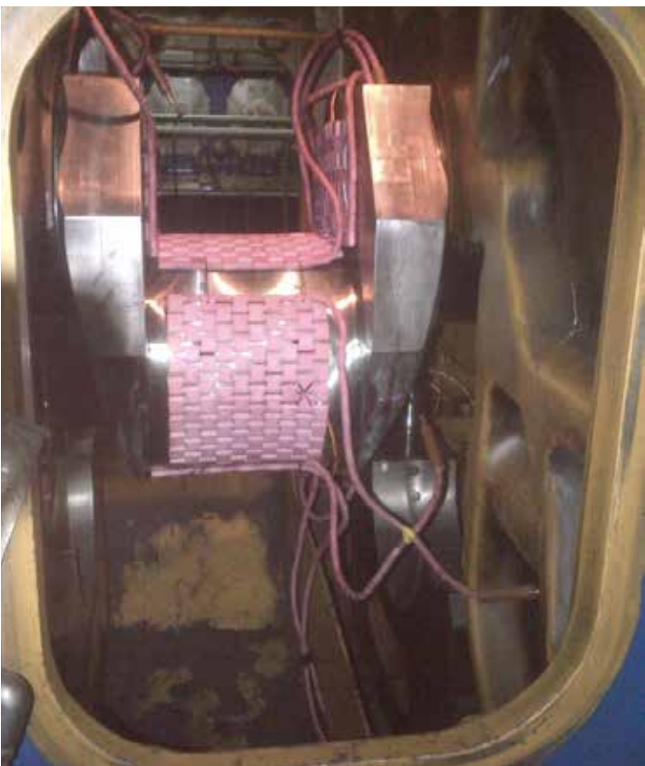
Annealing pads installed on damaged crankpin
