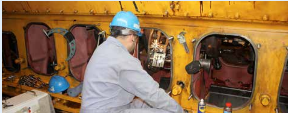
Post Annealing crankpin machining
