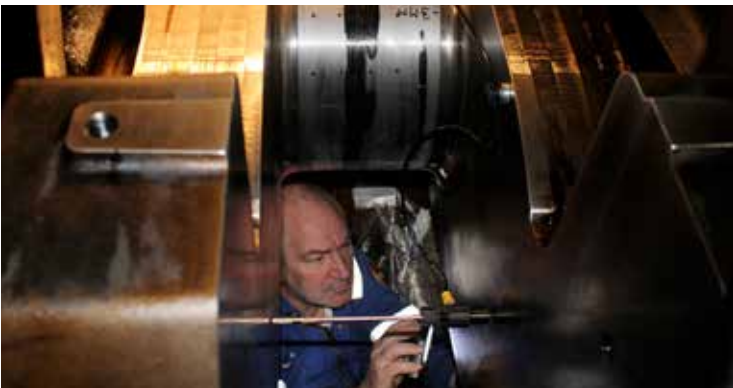
Checking deflection at -3mm (high hardness areas visible on center and right side of crankpin journal)
