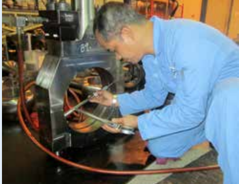
Calibration checks on big end bearing housing
