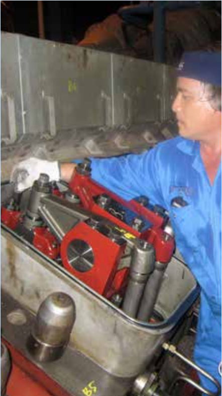
Installation of cylinder head
