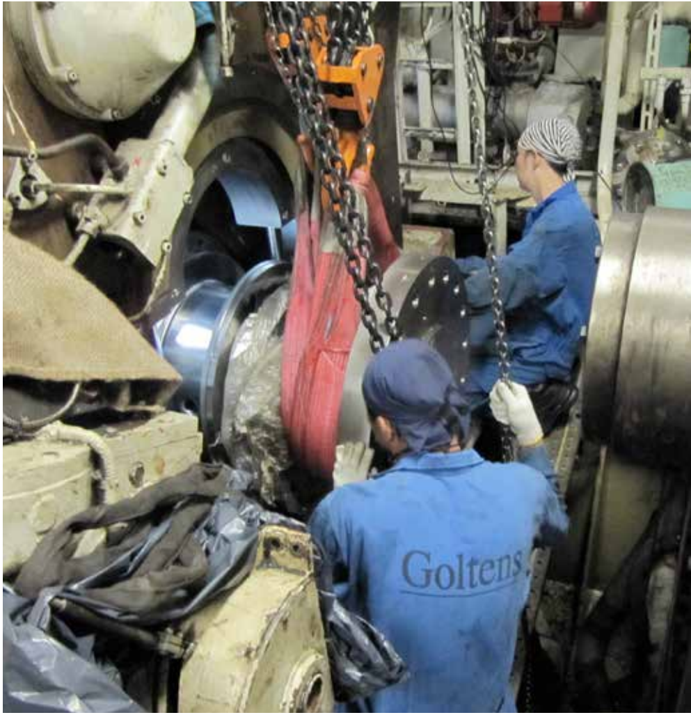
Maneuvering crankshaft into position
