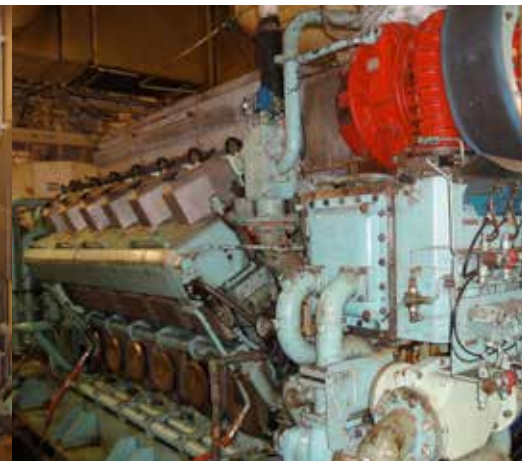
One of the completely overhauled and fully tested Wartsila engines type 12V22MD
