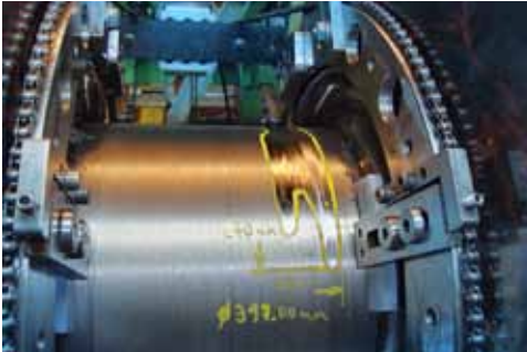
High hardness areas visible on right side of journal after baseline machining
