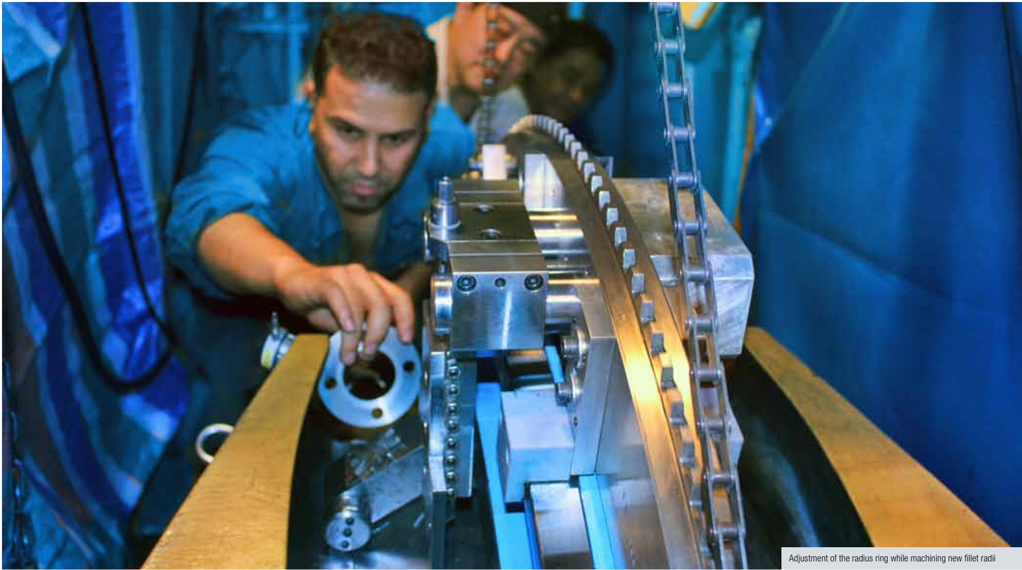
Adjustment of the radius ring while machining new fillet radii
