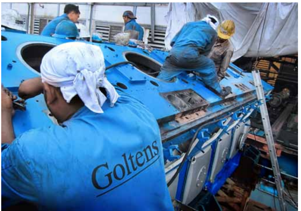
Cleaning and re-tapping all the threaded holes
