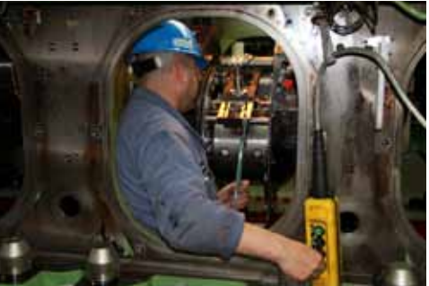
Machining the crankpin journal after annealing
