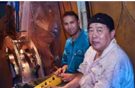
Single point cutting tools installed on damaged journal
