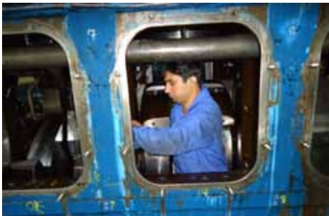
Installation of a wireless crankpin bearing sensor
