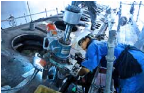
Modification of the fuel pump mounting
