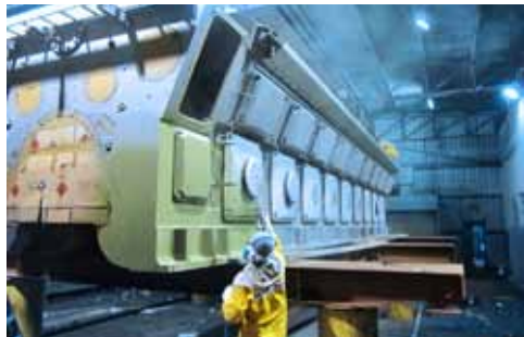
Primer coating after full sandblasting
