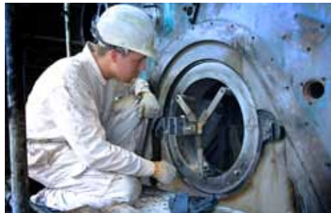
Laser alignment inspection of the main bearing pockets
