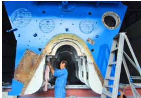
Inspection of bearing saddle landing surfaces
