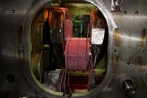
Ceramic heating tiles mounted to damaged journal prior to annealing
