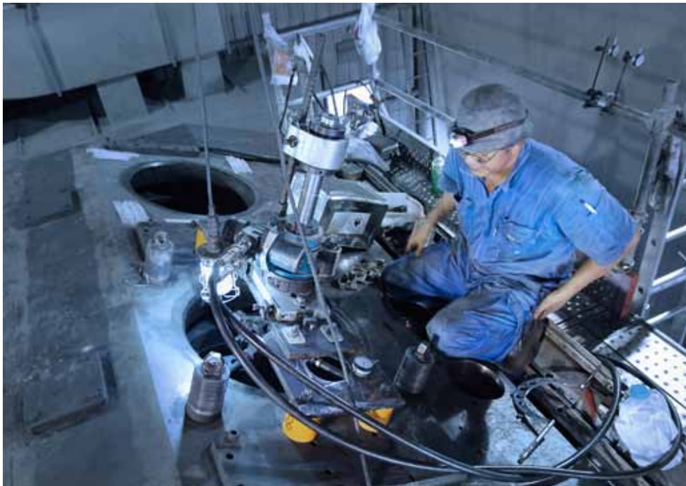
Boring of the lower liner seating area and installation of a bushing
