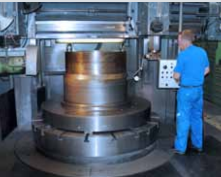
Machining horizontal surfaces of a 7-ton bear head to within 0.02mm tolerance
