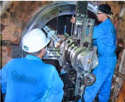
Boring of the stinger hinge to 1350mm
