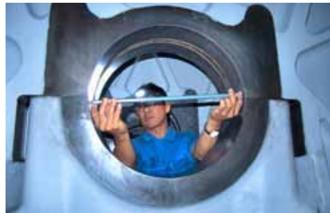
Calibration of main bearing pockets
