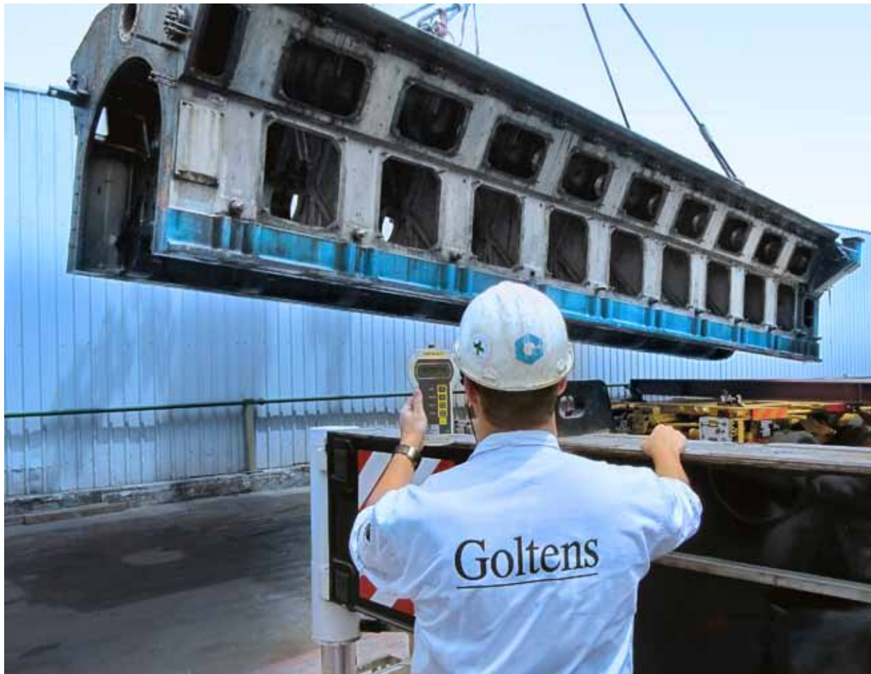
Offloading the engine block in the Goltens Singapore workshop, using a mobile crane
