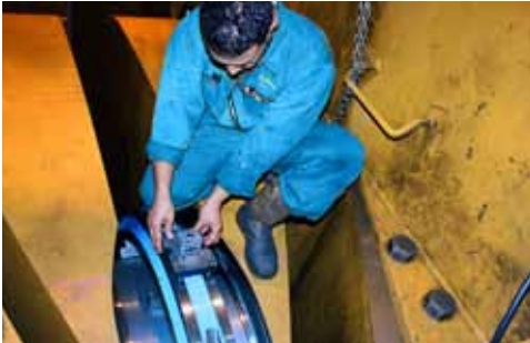
Installation of the radius ring prior to fillet machining
