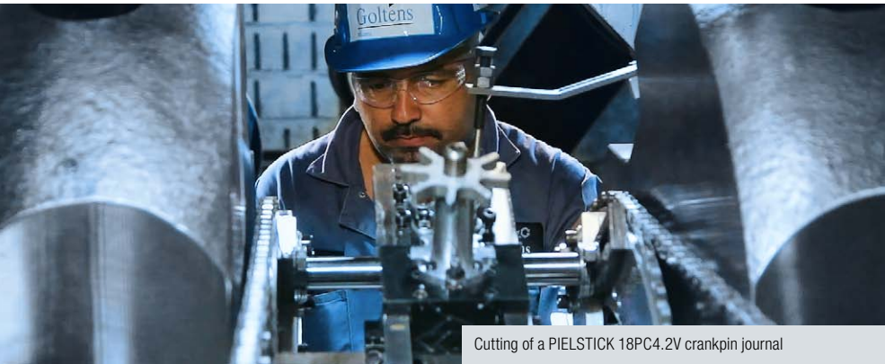
Cutting of a PIELSTICK 18PC4.2V crankpin journal
