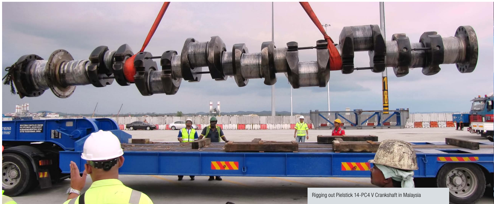
Rigging out Pielstick 14-PC4 V Crankshaft in Malaysia
