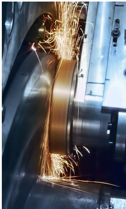
In-situ grinding of damaged thrust collar surface
