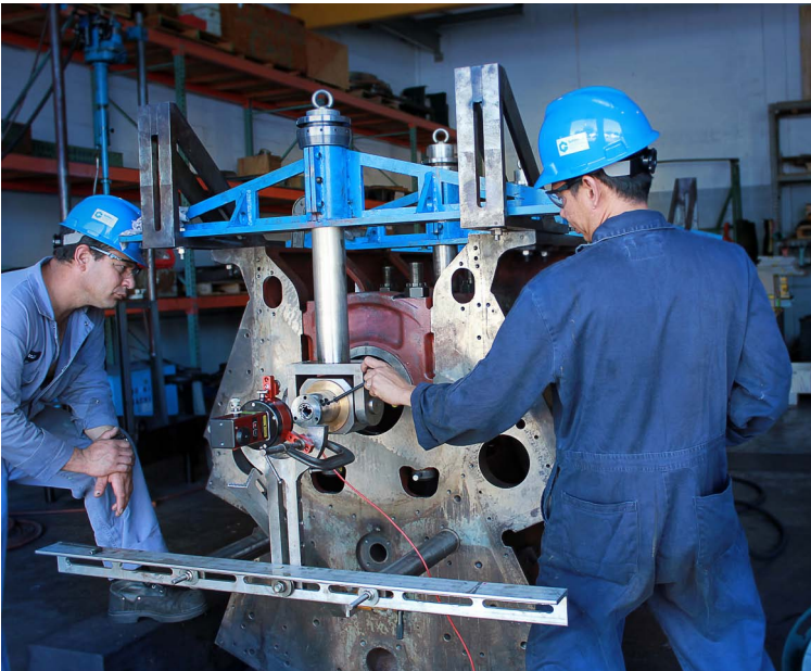
Laser Alignment of Line Boring bar prior to cutting
