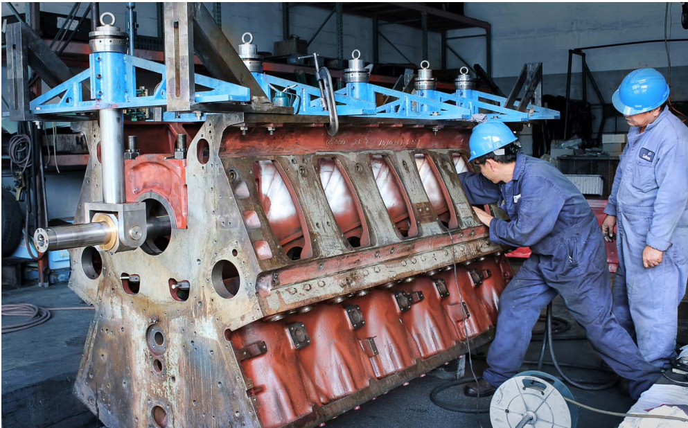
Making adjustments to the Line Boring equipment during boring
