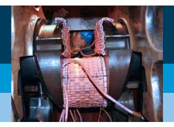
Over the past 5 years, Goltens stations around the world have successfully annealed over 75 crankshafts, saving customers tens of millions of dollars in unnecessary crankshaft purchases, major engine rebuilds, as well as countless days of lost operational capacity.
