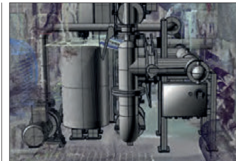
Optimarin Ballast System model overlaid on 3D scan results.
