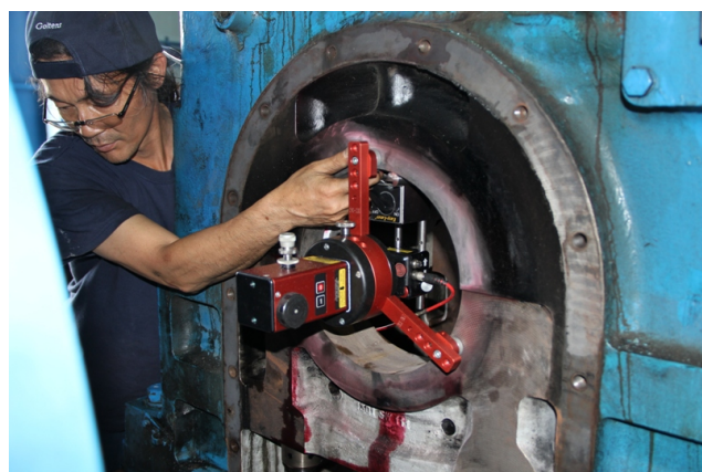
Laser Alignment check of bore prior to Line Boring
