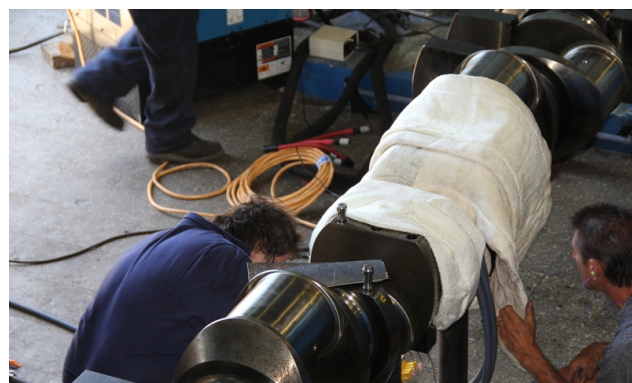
Induction Annealing Equipment being set up
