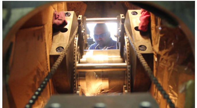
Grinding of crankpin In-Situ
