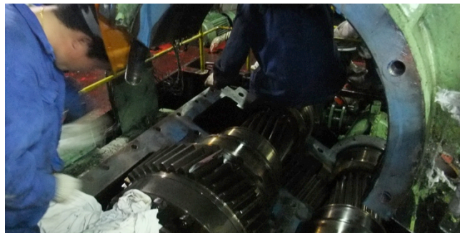
Overhaul of Main Engine Gear Box
