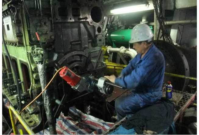
Workshop crankshaft grinding
