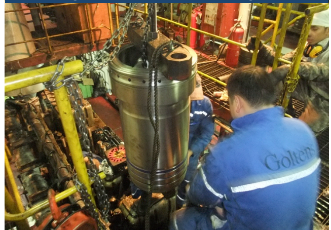
Rebuilding the Yanmar 6N330 main engine
