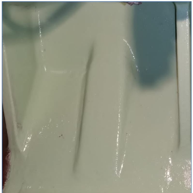
Figure 5: Metal stitched area after painting
