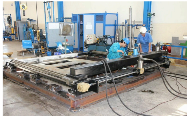
X-Y Milling of cooler box plate in Goltens' shop
