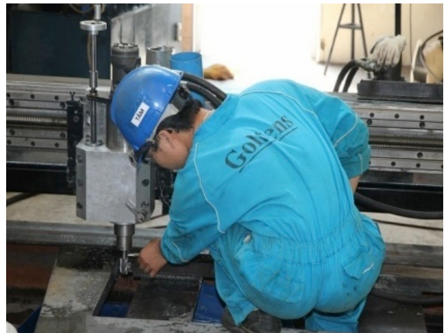
X-Y Milling of cooler box plate in Goltens' shop
