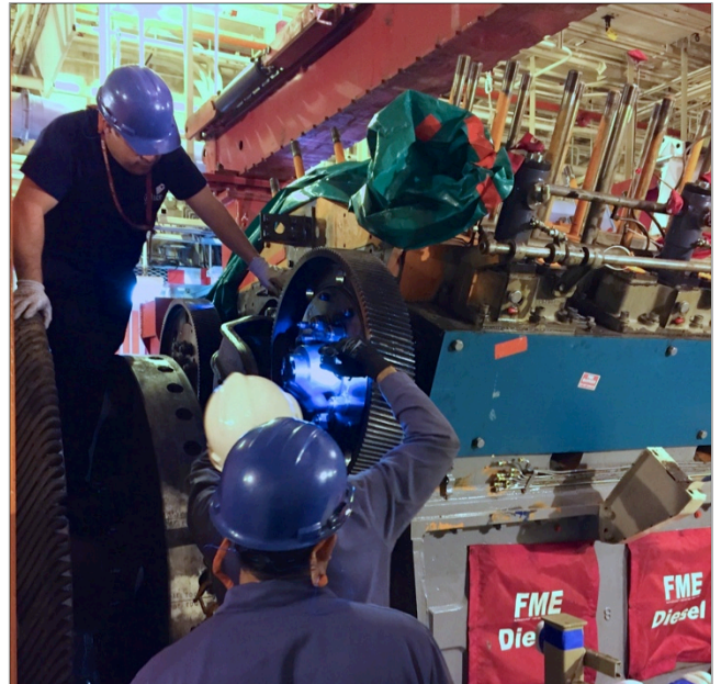
Disassembly and removal of gear train
