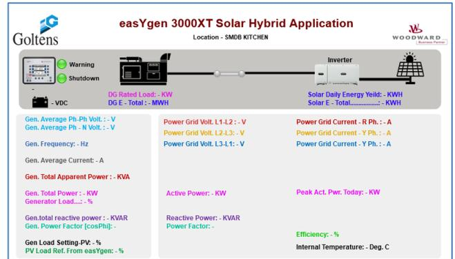
Figure 1: Remote Monitoring – System Status
