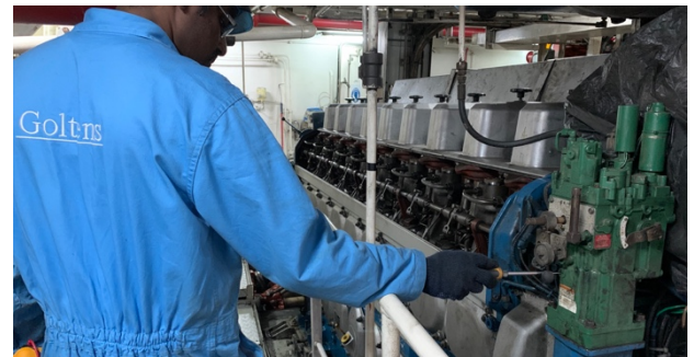
Figure 1: Woodward 3161 installation before upgrade
