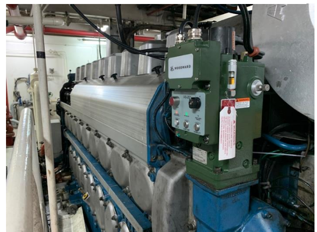
Figure 3: Woodward UG25+P3 after retrofit
