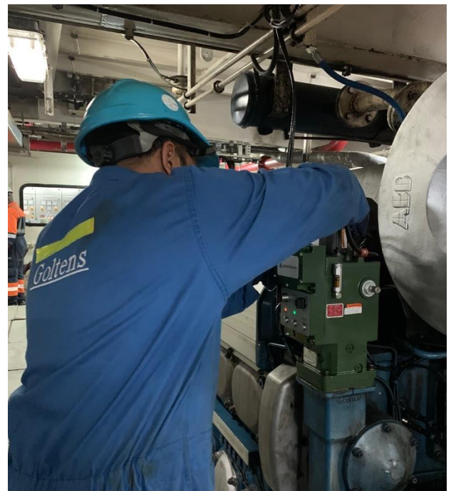
Figure 2: Technician fitting the Woodward UG25+P3
