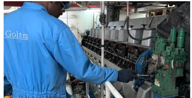
Figure 1: Woodward 3161 installation before upgrade
