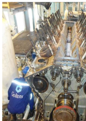
Laser Alignment check of engine bore
