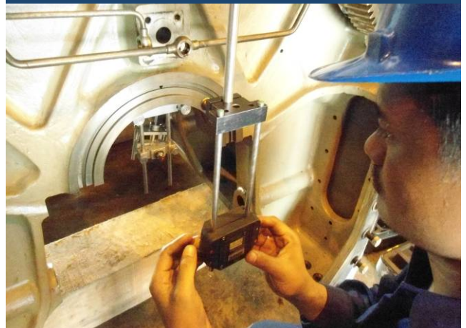
Laser Alignment check of engine bore
