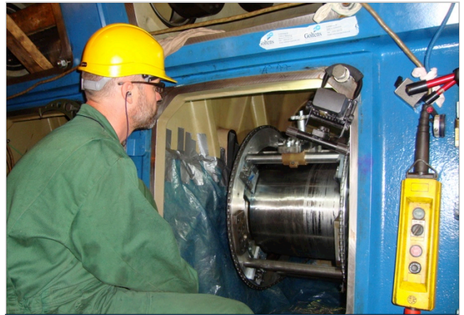
Pre-machining to remove cracks before annealing
