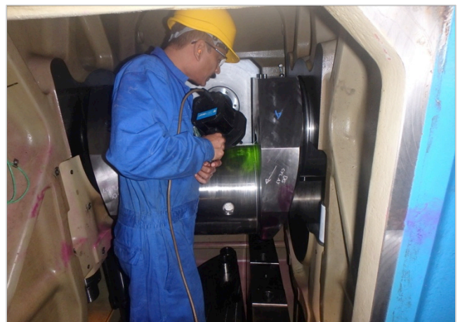
Crack tests performed on Crankpin #7
