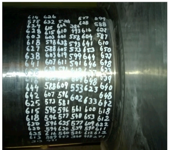
Hardness map showing extent of damage
