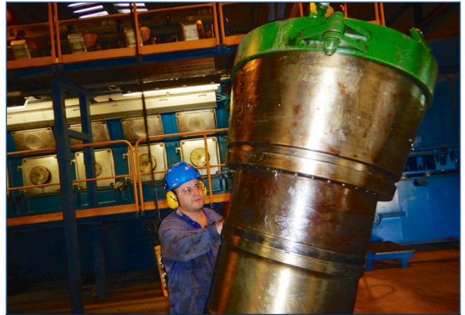
Rigging of honed liner into position
