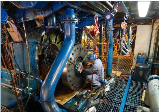
Removal of Vibration Dampener
