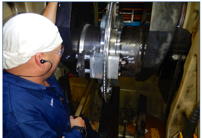
Machining new fillet radii after annealing
