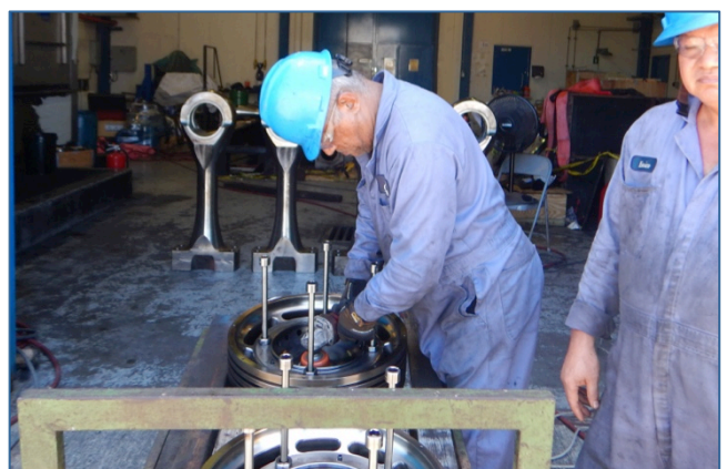
Calibration and overhaul of pistons
