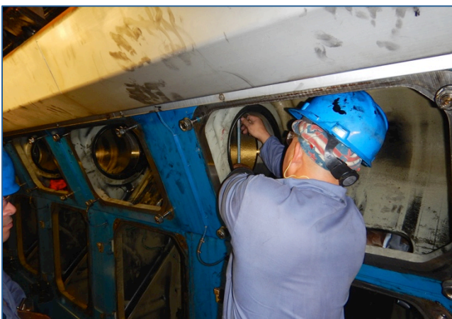
Calibration check on camshaft bores
