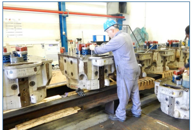
Overhaul of cylinder heads in powerhouse
