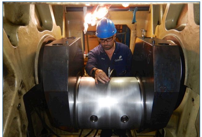
Calibration check after in-place machining
