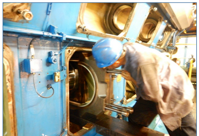
Installation of big end bearing housing
