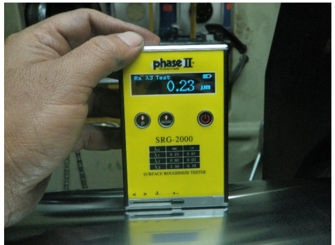
Final surface roughness 0.23Ra
