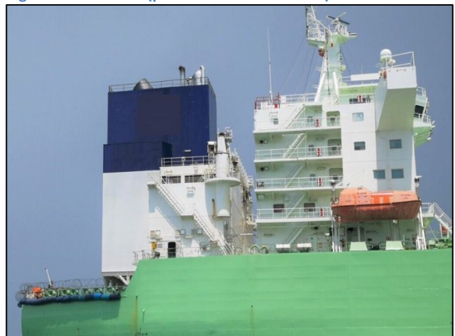
Figure 3: Extended funnel with scrubber installed
