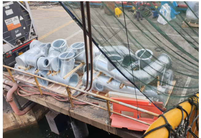
Figure 4: Prefabricated Big Bore Pipe supplied by Goltens
