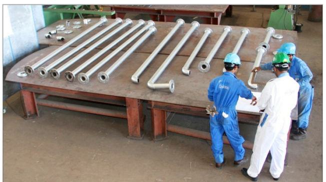
Prefabrication of system piping according to drawings
