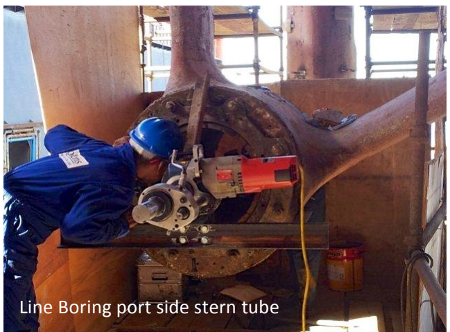
Calibration checks on stern tube to determine ovality/extent of damage
