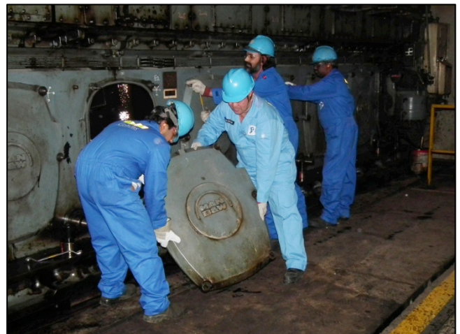
Disassembly of one of the MAN B&W engines
