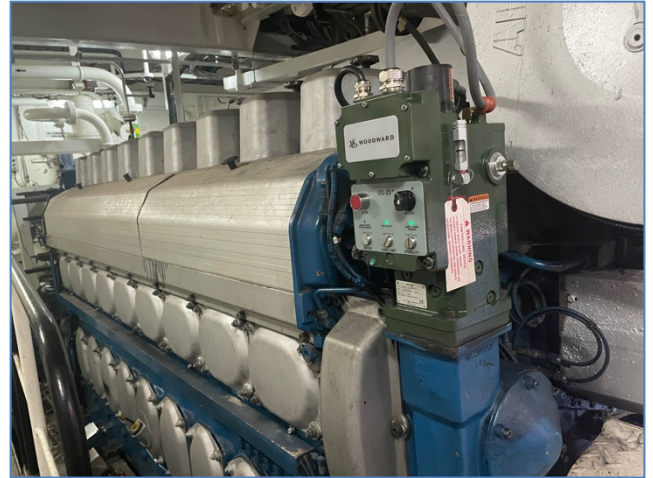
Figure 4: Woodward UG25+P3 installed on Wartsila 9L20
