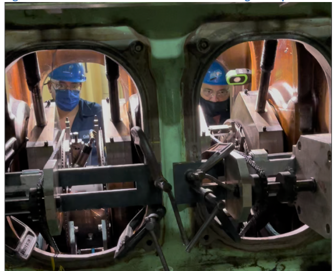
Figure 2: Simultaneous machining of crankpins 3 and 4
