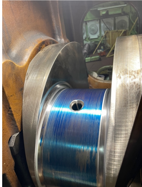
Figure 5: Blue fitting of crankpin journal surface to verify proper contact
