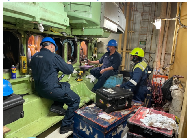
Figure 3: Machining crankpin #6 under observation of ship's crew
