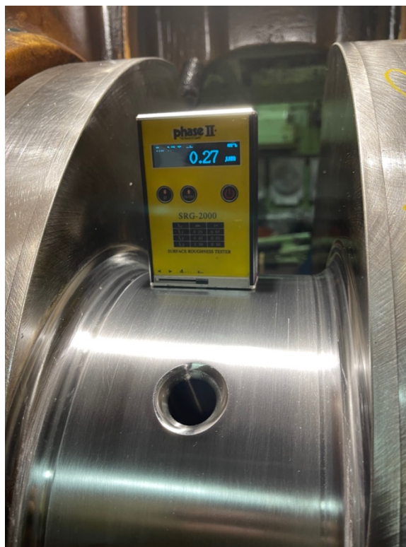
Figure 6: Final check of surface roughness on crankpin journal found within limits
