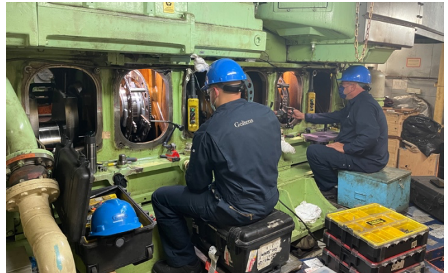
Figure 1: Goltens' In-Place Machinists machining crankpins 2 & 5
