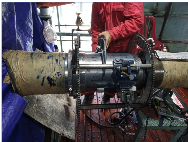
Figure 2: Measurement of undercut shaft at (3.30mm)
