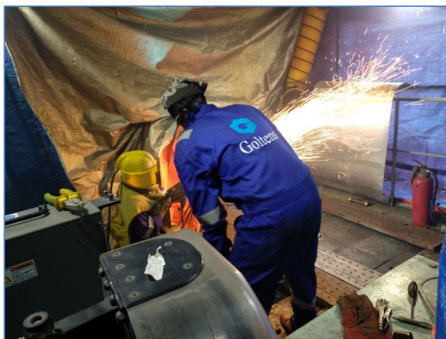
Figure 3: Remetalling/Thermal Spraying of agitator shaft
