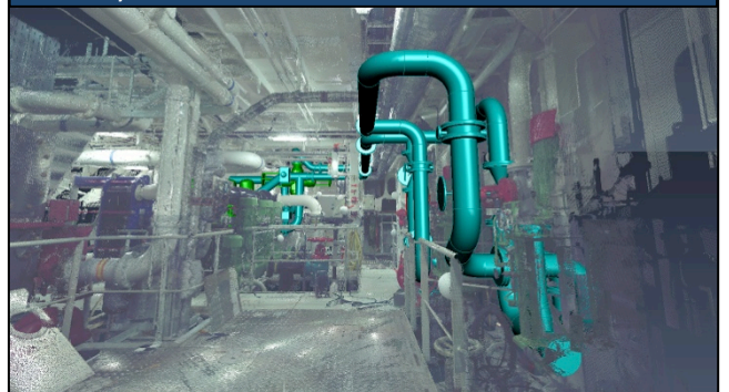
BWT System overlaid on 3D scan results
