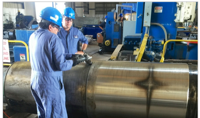
Preparing rudderstock for tool installation
