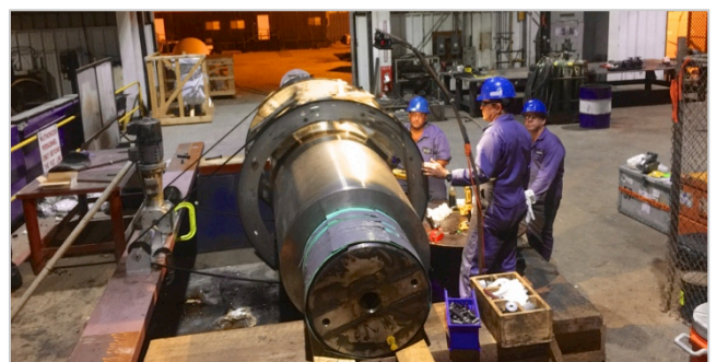
Journal Machining in progress
