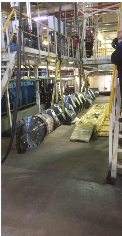
Rigging new crankshaft
