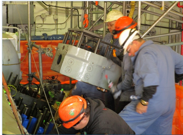
Installation of cylinder heads prior to testing
