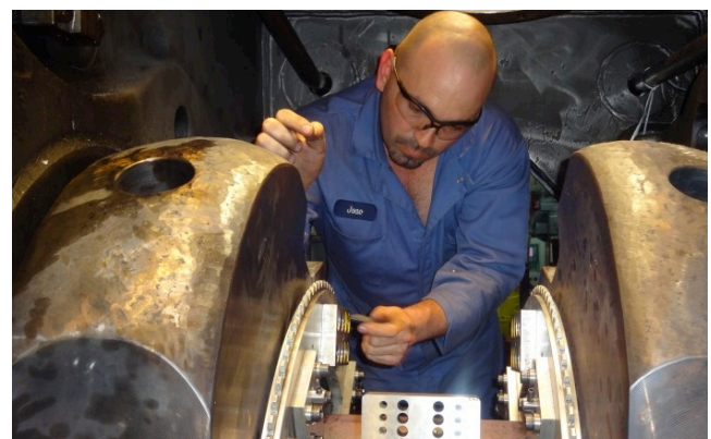
Setting up tooling for post annealing machining
