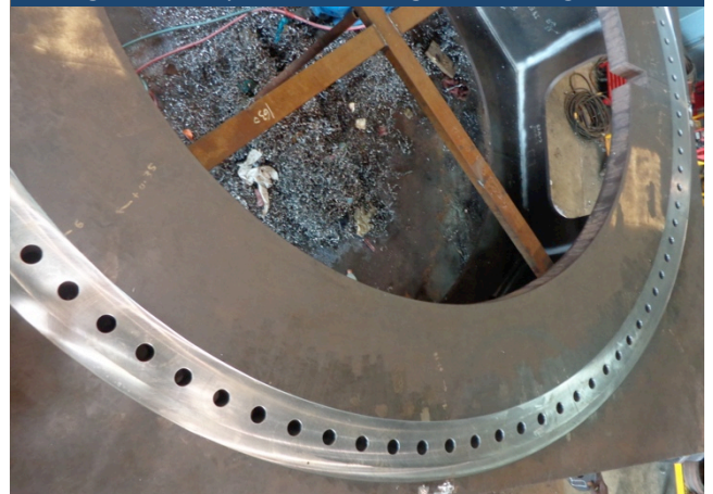
Flange surface post machining and drilling
