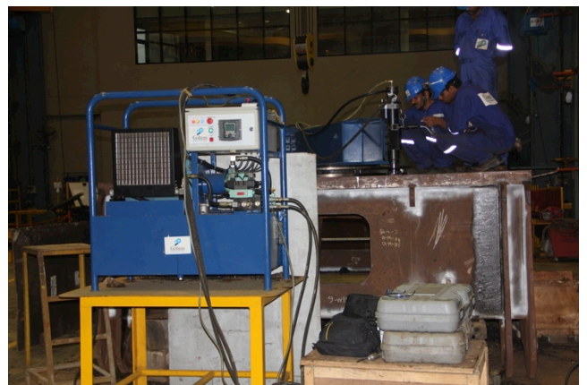
Flange surface post machining and drilling
