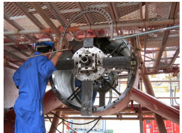
One of the Six thruster housings machined
