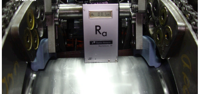
Completed crankpin journal with surface finish <math><0.2R_a</math>
