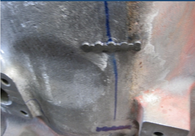
Lock hammered into position
