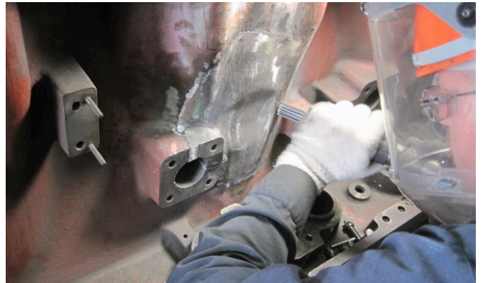
Finishing the completed stitch and preparing for the lock
