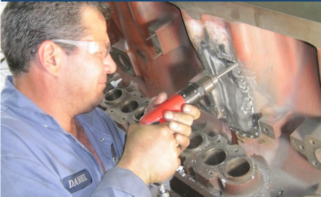
Drilling the hole pattern for the lock insert
