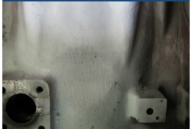
Completed repair – no cracks present
