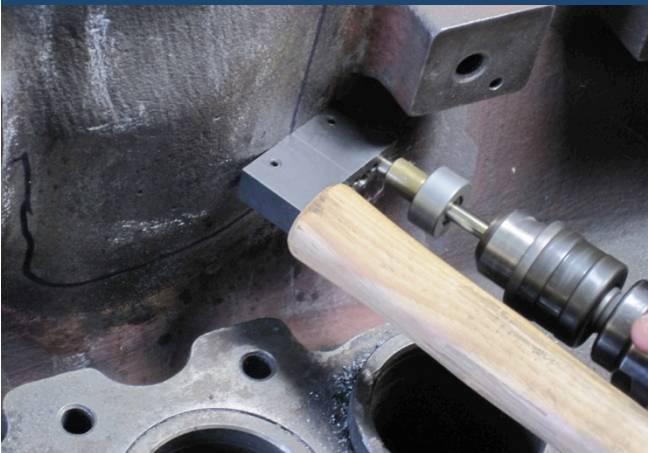
Lock hammered into position
