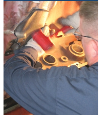
Stitching bolts in place along the seam
