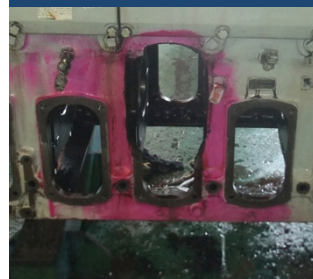
Metal stitching of replacement door to block
