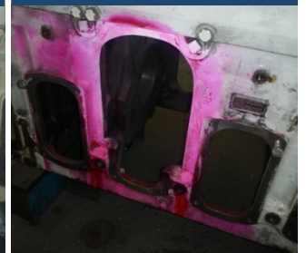
Metal stitching of replacement door to block
