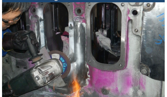
Dye penetrant crack test of repaired block
