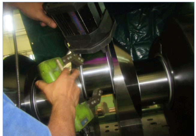
MPI crack tests performed on all journals
