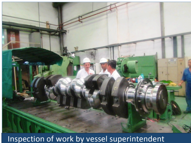
Calibration check on main bearing pockets
