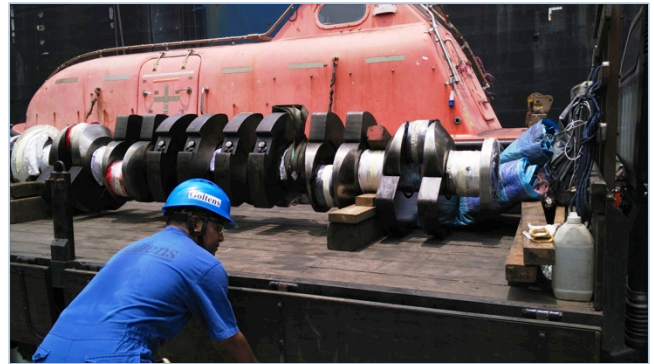
Damaged crankshaft rigged for transport to shop
