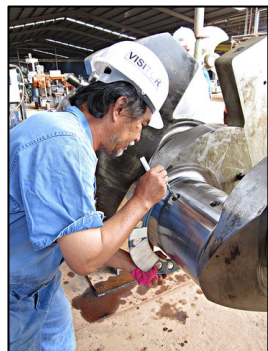
Bore alignment and crankshaft calibration
