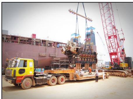
Rigging of the engine block ashore
