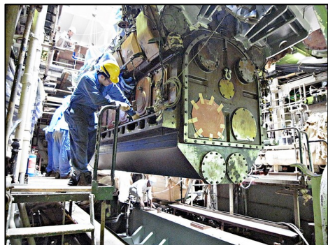
Lowering the engine into position
