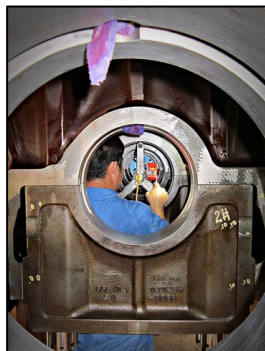
Bore alignment and crankshaft calibration
