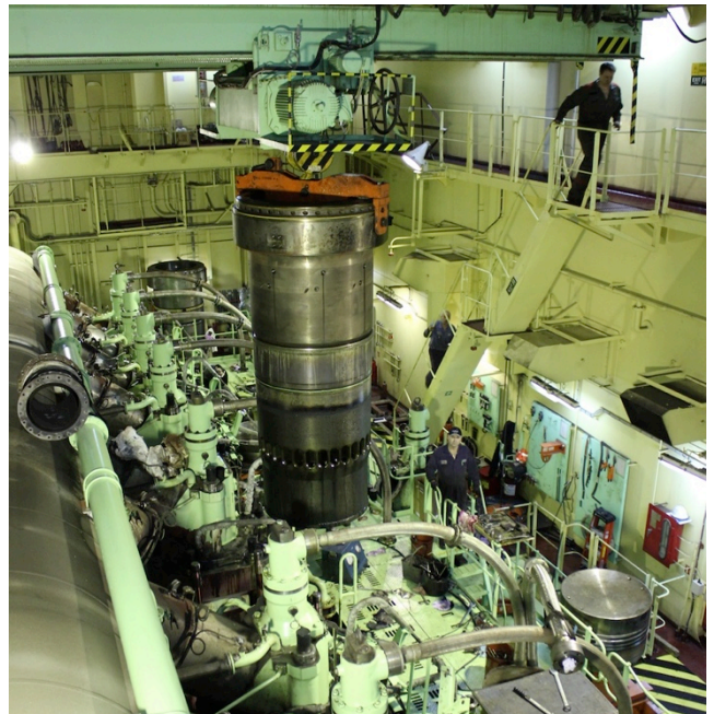
Worn liner being removed from the engine
