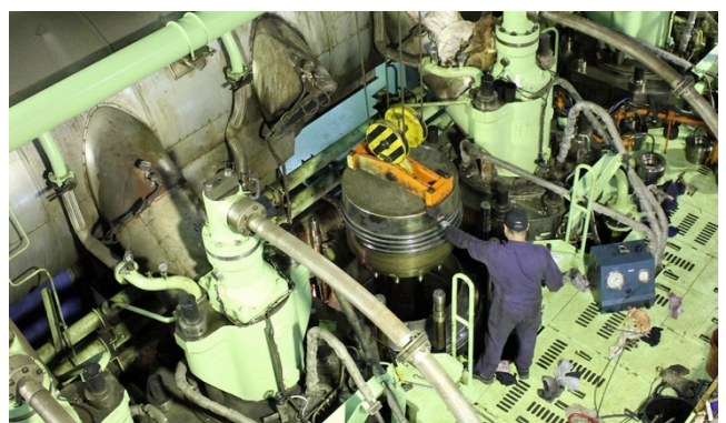
Installation of overhauled piston
