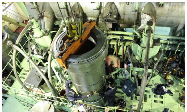
Replacement liner prepared for installation
