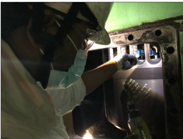
Figure 5: Adjusting LDM position on top of piston
