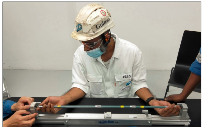
Figure 3: LDM calibration prior to measurement
