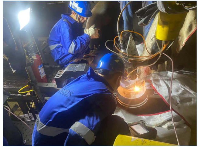
Laser cladding of bearing housing
