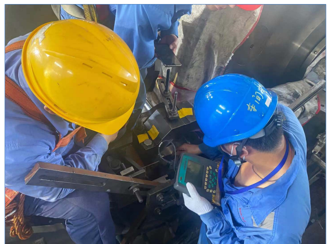
Hardness and calibration checks after machining
