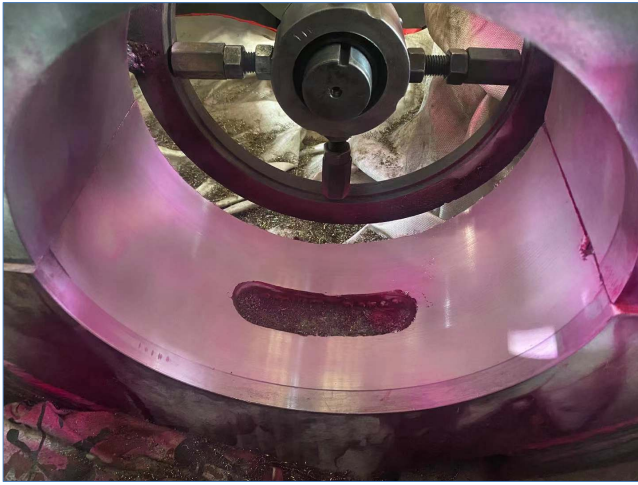
Dye-check of bearing housing inner surface before laser cladding
