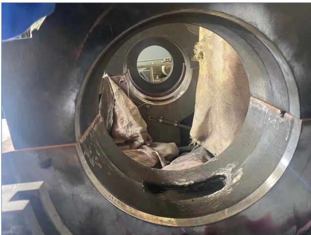
Inner housing surface after laser cladding
