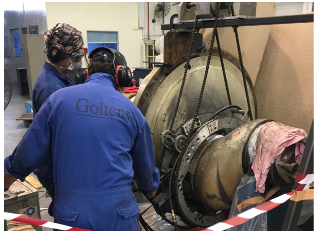
Figure 2: Removing cracks and hardness before cladding
