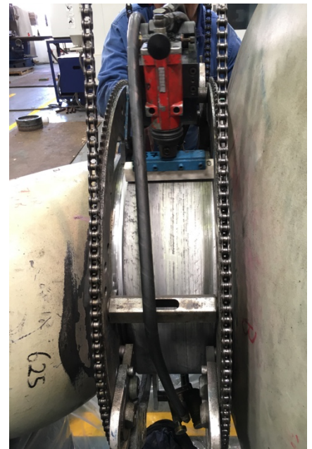
Figure 6: Machine honing to finish diameter
