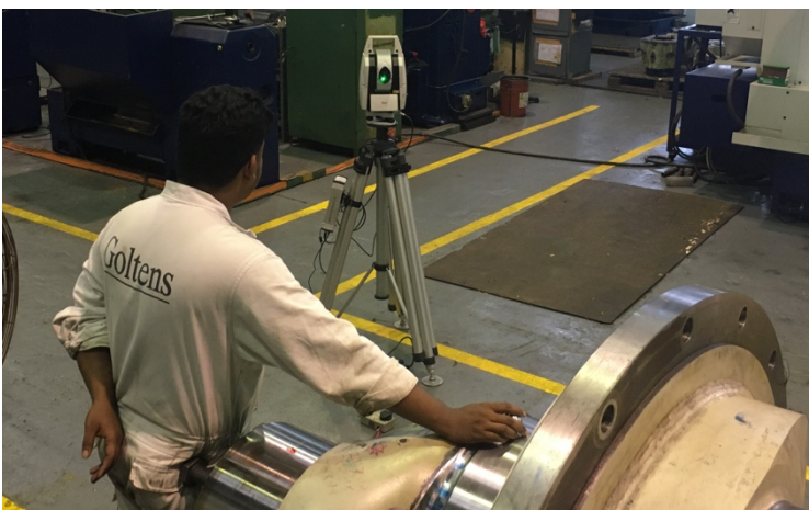
Figure 9: Final inspection with portable CMM (Leica Laser Tracker)
