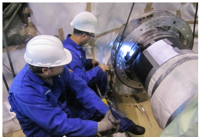
Turbine journal machining in progress
