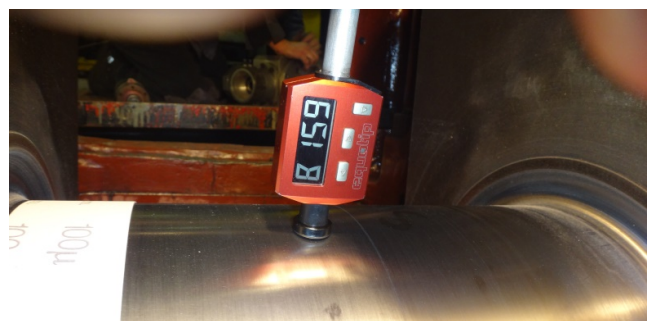
Performing hardness checks on damaged journal
