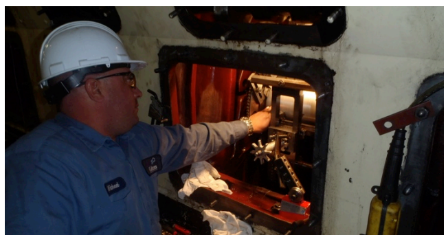
Adjusting Goltens' Single Point Cutting Tools
