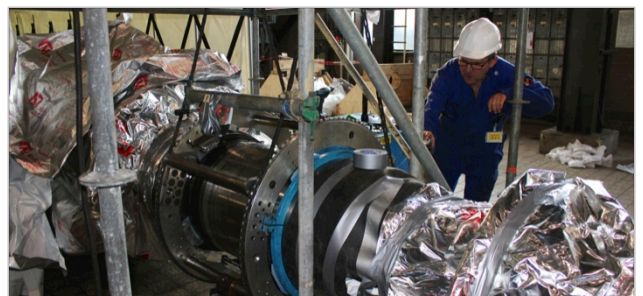
Machining of the damaged rotor shaft in progress
