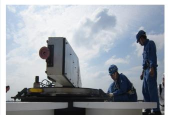
Adjusting Goltens' 6 meter flange facing machine on the chain table surface prior to machining
