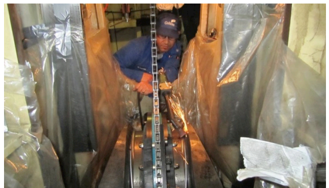
Machining of new fillet radii
