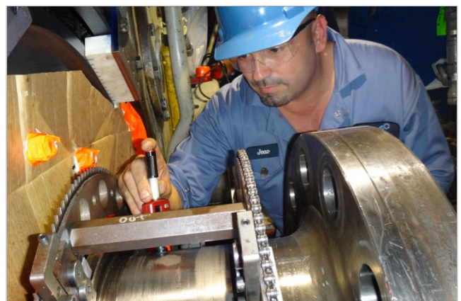
Hardness checks during pre-annealing machining
