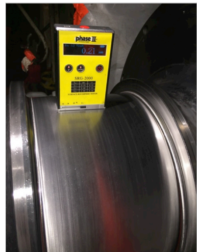
Finished surface at 0.21\text{ Ra}
