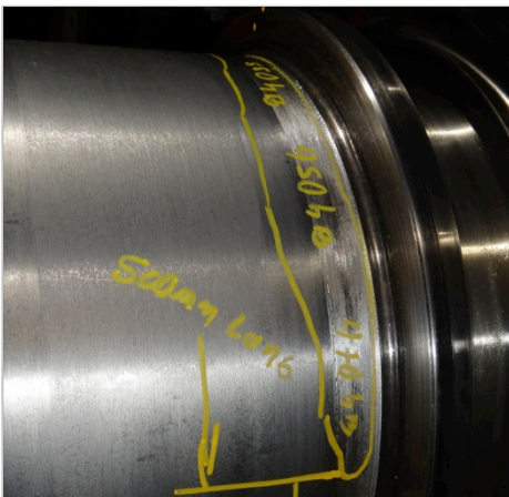
Surface hardness at -2.00\text{mm}
