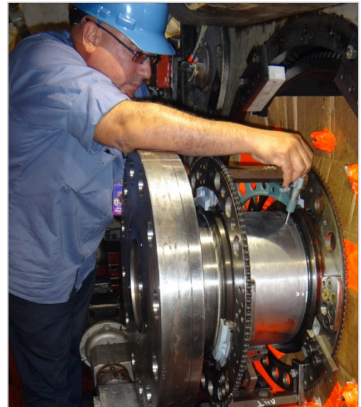
Checking shaft diameter pre-annealing
