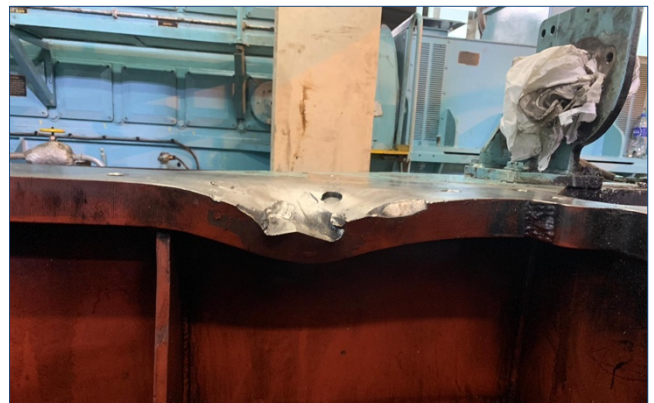
Figure 3: Bedplate damage from component impact
