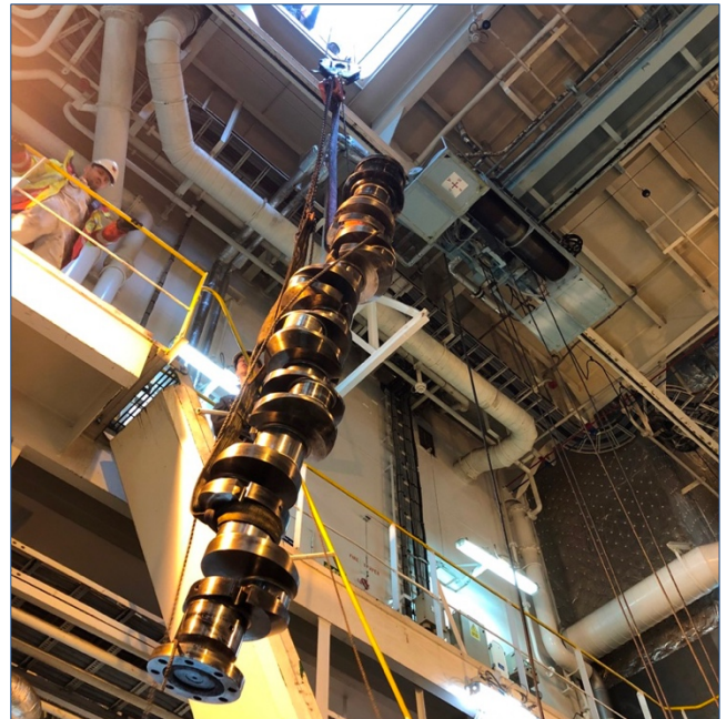
Figure 2: Rigging condemned crankshaft from engine room
