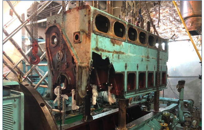
Figure 1: Damaged engine disassembled and jacked
