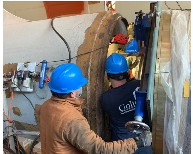
Figure 3: Utilizing diamond grinding Discs to remove tungsten surface layer.
