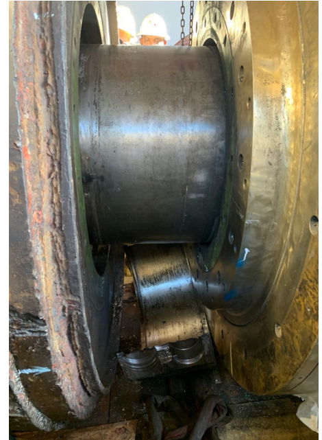
Figure 6: Shaft after liner removal
