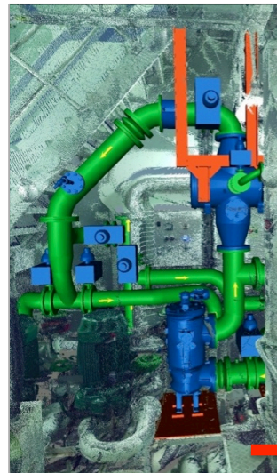
Hyde Guardian System modeled on 3D Scan output
