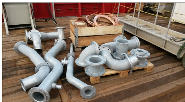
Sections of pre-fabricated/pre-galvanized piping kit
